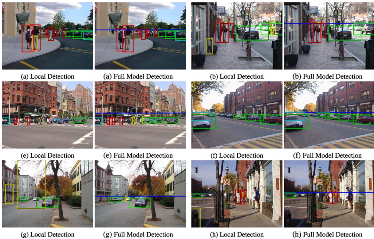
Fig. 11 (Color online) We show local object detections ( left ) of Dalal-Triggs ( green = true car, cyan = false car, red = true ped, yellow = false ped) and the final detections ( right ) and horizon estimates ( blue line ) after considering surface geometry and camera viewpoint (initially estimated using our example-based method). Our method provides large improvement (+7%/11% for peds/cars at 1 FP/image) over a very good local detector. Many of the remaining recorded “false
