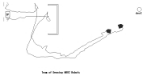
Figure 9: Teleautonomous extrication from a box canyon of a team of 2 Denning mobile robots (viewed from above).
