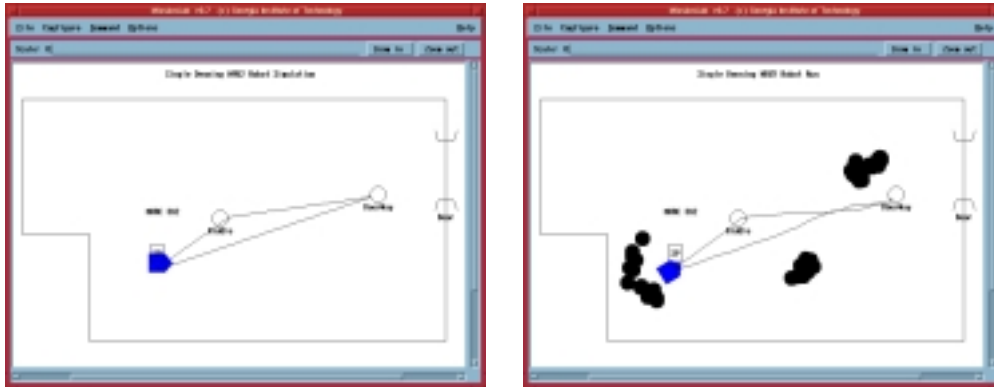
Figure 7: Left: Simulated Run on Denning Robot. Right: same code executed on actual Denning Robot
