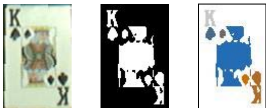
Figures 10-12: Images of king of spades: raw (left), binarized (middle), regions colored (right)
