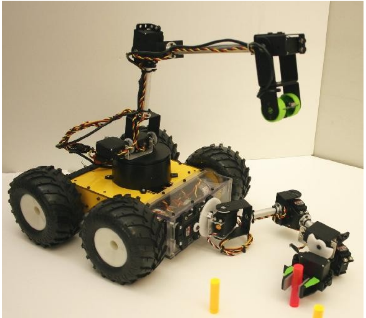
Regis: 4DOF “goose neck”: base (pan), shoulder/elbow/wrist (tilt)
