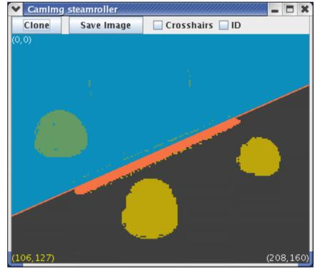
Subtle point: bool overrides uchar in the SketchGUI, so selecting yellow\_stuff allows the top yellow blob to display even though the inverted (orange) *topside* is covering its appearance in *camFrame*. (Competing bools are averaged.)
