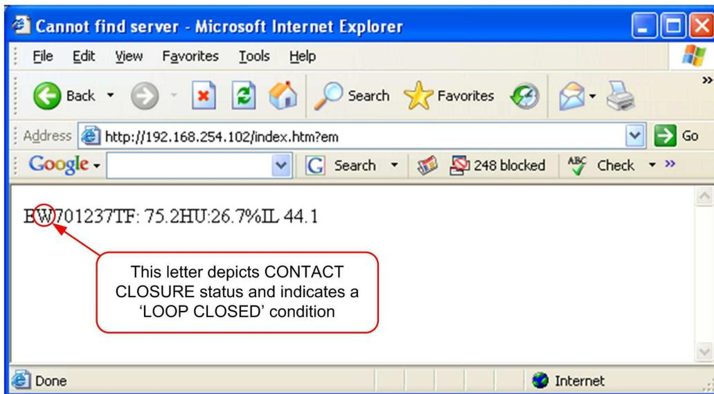
Figure 12 Valid Contact Closure status showing switch closed after resetting.
