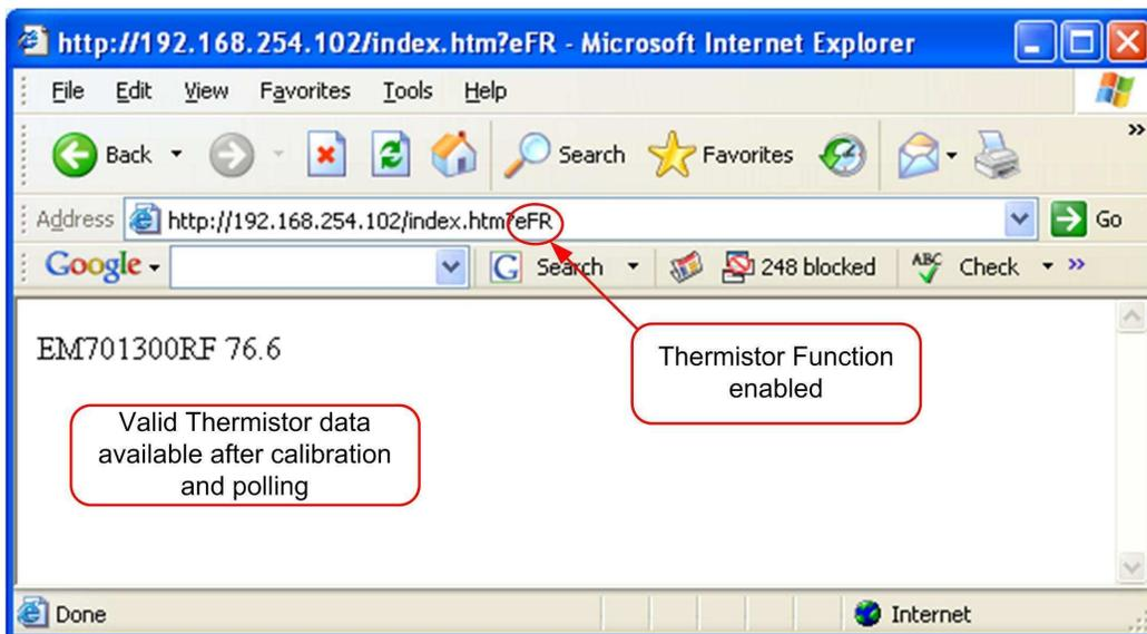
Figure 14 Command used to enable Thermistor function.
