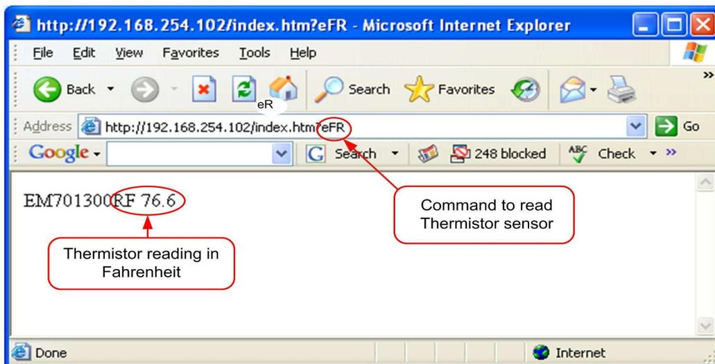
Figure 17 - How to obtain a Thermistor reading.
