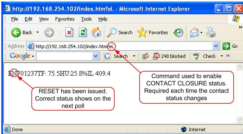
Figure 11 Contact Closure RESET command issued
