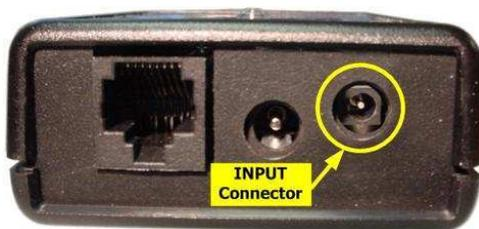
Figure 7 – Thermistor, Voltage Measurement and Contact Closure input connector.
