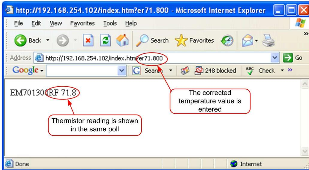
Figure 16 - Calibration temperature is entered.
