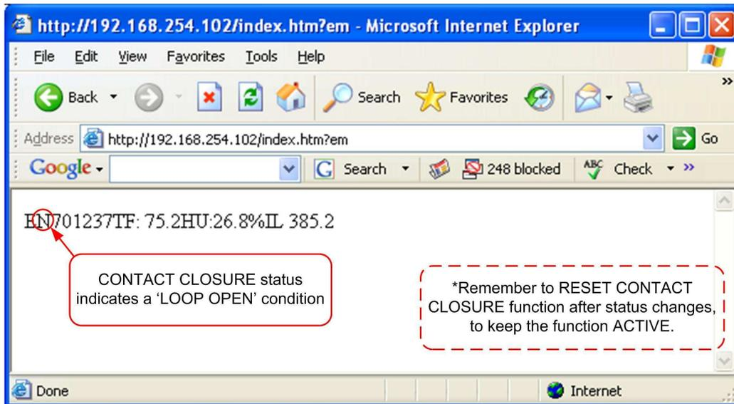
Figure 13 Open switch or open loop indication.
