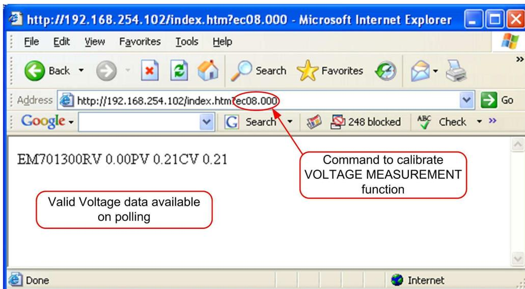
Figure 19 - Command to calibrate DC Voltage Measurement.
