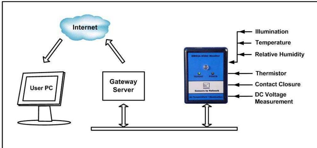
Figure 2 – How Websensor works.
