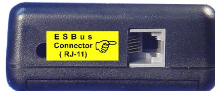
Figure 6 - Eibus Connector (RJ-11).
