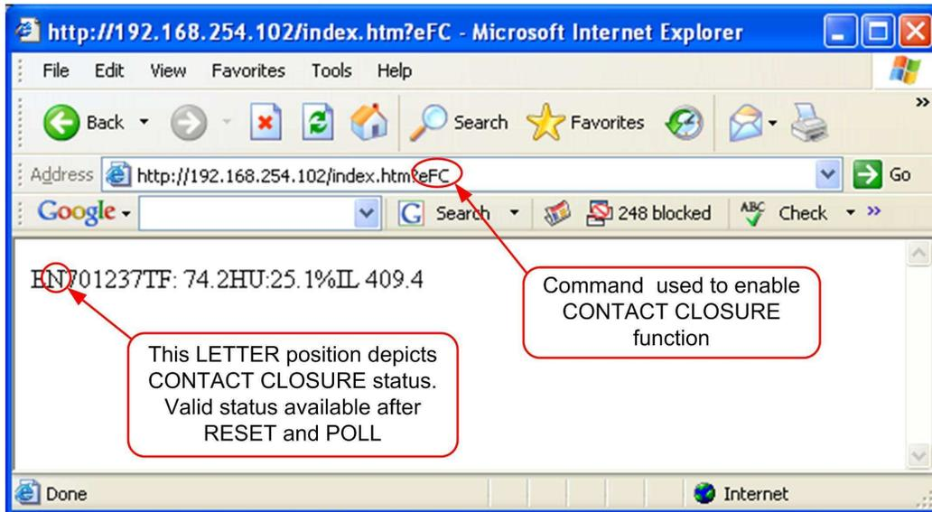
Figure 10 - Command enabling Contact Closure
