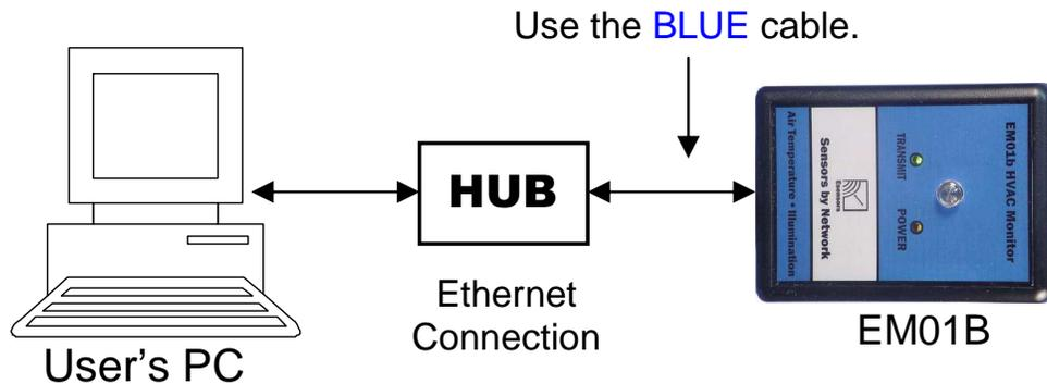
Figure 4 - Websensor connected through a HUB to the NIC in a PC.
