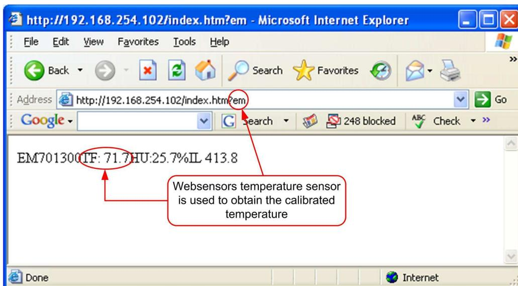
Figure 15 - Using Websensors own temperature for calibration.
