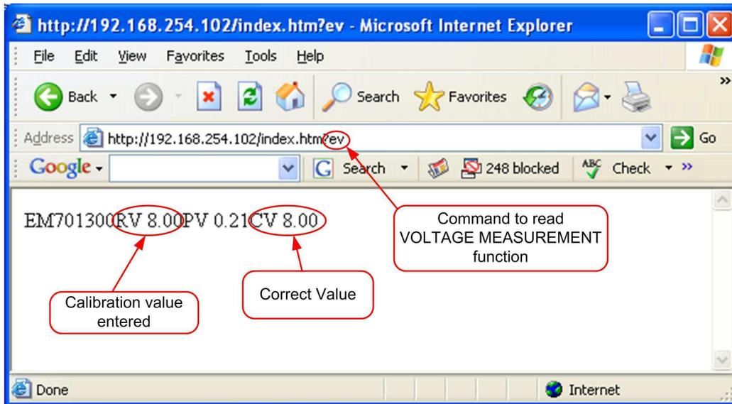
Figure 20 - Command to Measure DC Voltage.
