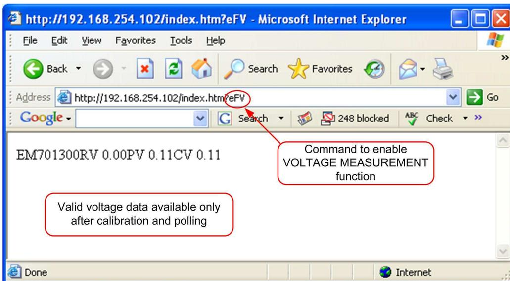
Figure 18 - Command to enable DC Voltage Measurement.
