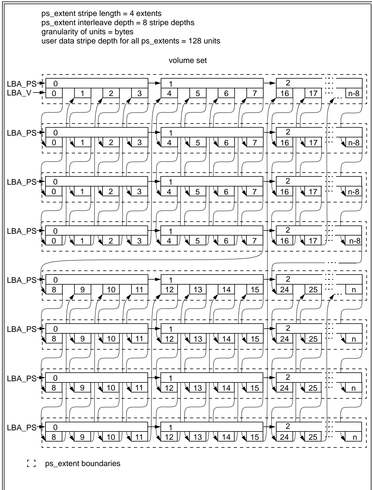
Figure C.5 - User data mapping for a RAID 3 configuration
