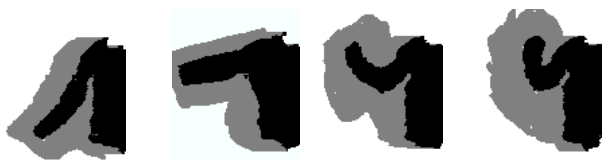
Figure 5: Examples of pose templates. The excitatory region is shown in black and the inhibitory in gray. White regions are not considered in the matching process.
