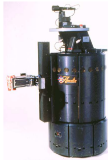
Figure 1: AMELIA, the robot used in our research, is a RWI B21 robot equipped with a color camera mounted on a pan-tilt unit, 24 sonar sensors, and a 180° SICK laser range finder.
