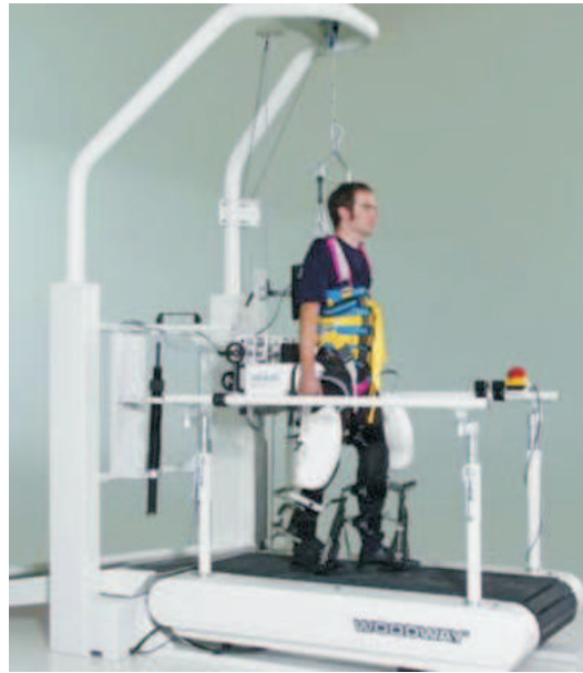
Figure 6.3. Example of orthotic device for gait rehabilitation. The 'Lokomat' has been developed at the ParaCare Research Laboratory (Prof. V. Dietz) of the University Hospital Balgrist, University of Zurich, Switzerland, in collaboration with the Institute for Automatization (Prof. M. Morari) of the Swiss Federal Institute of Technology (ETH), Zurich, Switzerland, and is now commercialized by the HOCOMA AG (picture courtesy of the ParaCare Research Laboratory).
