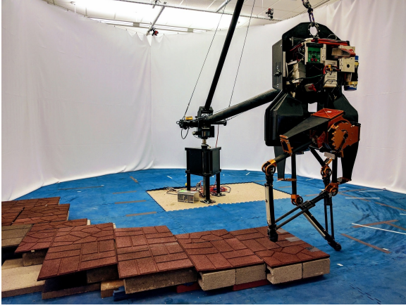
Fig. 1. CMU's ATRIAS biped shown in the boom testbed during the ground disturbance experiments with unexpected height changes of \pm 15 cm (discussed in section IV-C).
