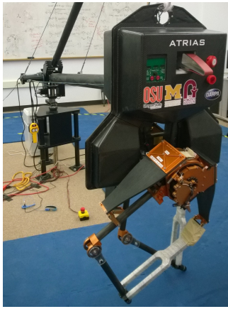
Fig. 9. CMU's copy of ATRIAS [28], currently mounted on a boom to validate planar running using the deadbeat leg placement policy from the SMM.
