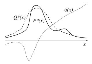
Figure 2. Functions involved in importance sampling. We wish to estimate the expectation of  $\phi(x)$  under  $P(x) \propto P^*(x)$ . We can generate samples from the simpler distribution  $Q(x) \propto Q^*(x)$ . We can evaluate  $Q^*$  and  $P^*$  at any point.
