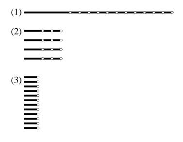
Figure 13. Three possible Markov Chain Monte Carlo strategies for obtaining twelve samples using a fixed amount of computer time. Computer time is represented by horizontal lines; samples by white circles. (1) A single run consisting of one long 'burn in' period followed by a sampling period. (2) Four medium-length runs with different initial conditions and a medium-length burn in period. (3) Twelve short runs.
