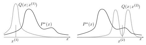
Figure 6. Metropolis method in one dimension. The proposal distribution Q(x';x) is here shown as having a shape that changes as x changes, though this is not typical of the proposal densities used in practice.
