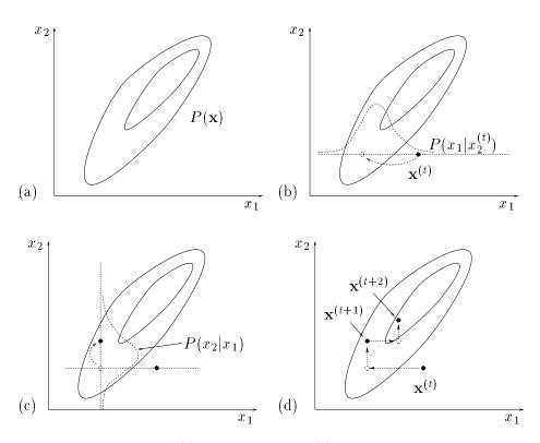
Figure 9. Gibbs sampling. (a) The joint density  $P(\mathbf{x})$  from which samples are required. (b) Starting from a state  $\mathbf{x}^{(t)}$ ,  $x_1$  is sampled from the conditional density  $P(x_1|x_2^{(t)})$ . (c) A sample is then made from the conditional density  $P(x_2|x_1)$ . (d) A couple of iterations of Gibbs sampling.
