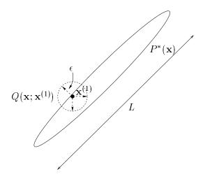
Figure 7. Metropolis method in two dimensions, showing a traditional proposal density that has a sufficiently small step size  $\epsilon$  that the acceptance frequency will be about 0.5.
