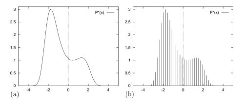
Figure 1. (a) The function  $P^*(x) = \exp\left[0.4(x-0.4)^2 - 0.08x^4\right]$ . How to draw samples from this density? (b) The function  $P^*(x)$  evaluated at a discrete set of uniformly spaced points  $\{x_i\}$ . How to draw samples from this discrete distribution?
