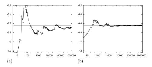
Figure 3. Importance sampling in action: a) using a Gaussian sampler density; b) using a Gaushy sampler density. Horizontal axis shows number of samples on a log scale. Vertical axis shows the estimate  $\hat{\Phi}$ . The horizontal line indicates the true value of  $\Phi$ .
