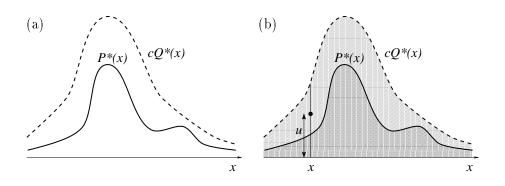
Figure 4. Rejection sampling. a) The functions involved in rejection sampling. We desire samples from  $P(x) \propto P^*(x)$ . We are able to draw samples from  $Q(x) \propto Q^*(x)$ , and we know a value c such that  $cQ^*(x) > P^*(x)$  for all x. b) A point (x, u) is generated at random in the lightly shaded area under the curve  $cQ^*(x)$ . If this point also lies below  $P^*(x)$  then it is accepted.
