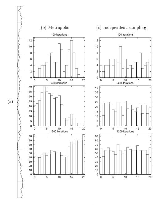
Figure 8. Metropolis method for a toy problem. (a) The state sequence for t = 1...600. Horizontal direction = states from 0 to 20; vertical direction = time from 1 to 600; the cross bars mark time intervals of duration 50. (b) Histogram of occupancy of the states after 100, 400 and 1200 iterations. (c) For comparison, histograms resulting when successive points are drawn *independently* from the target distribution.
