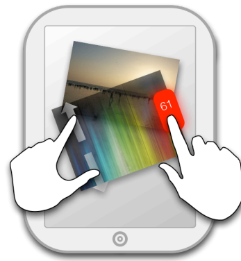
Figure 8: An illustration of a touchscreen-based application written with ConstraintJS. Constraints control the position, scale, and angle of photos, which users can manipulate with one or two fingers. When two fingers touch a photo, a red slider appears that controls the photo’s opacity and can be changed using a third finger. Constraints set the position and text of the slider.
