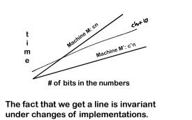
under changes of implementations. Different machines result in different slopes, but the time taken grows linearly as input size increases.
