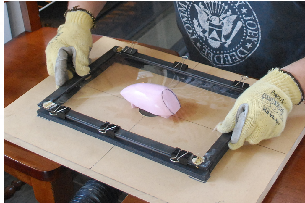
Making a canopy (windshield) for a model airplane.
