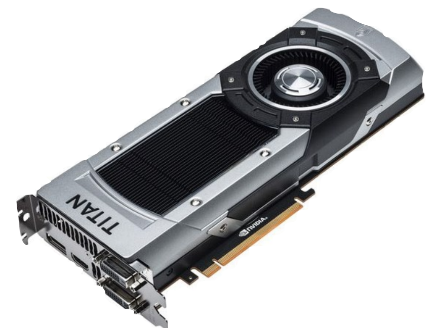
Titan X: 24 SMM cores (250 watts)
