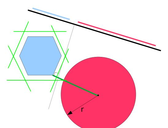
Separating axes to check are parallel to the edges of the polygon or the line joining the nearest vertex to the center of the circle.
