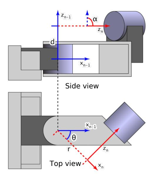
1) Move by d along  $z_{n-1}$ 2) Rotate by  $\theta$  around  $z_{n-1}$
