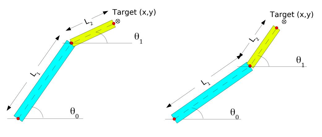
$s_{2}^{-} = -\sqrt{1-c_{2}^{2}}$  $\theta_{1}^{-} = \operatorname{atan2}(s_{2}^{-}, c_{2})$   $s_{2}^{+} = \sqrt{1-c_{2}^{2}}$  $\theta_{1}^{+} = \operatorname{atan2}(s_{2}^{+}, c_{2})$
