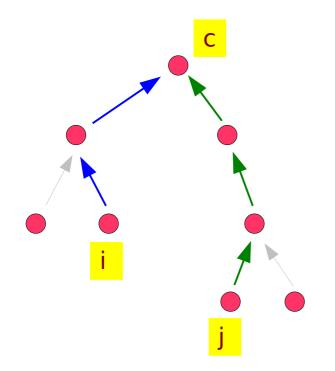
Search upward from i to common frame c, forming  $T_{ci}$ .
