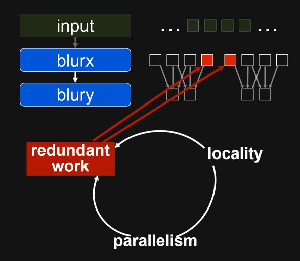
Stencil pipelines require tradeoffs determined by organization of computation
