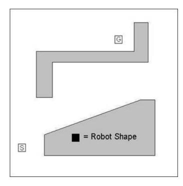
Use the following workspace (with robot shown at the start configuration), configuration space for a two link manipulator with no joint limits, and a distance between two configurations  $q_a$ and  $q_b$  given as:
