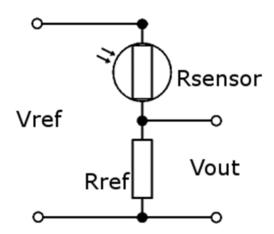
$$V_{out} = \frac{V_{ref} R_{ref}}{\left(R_{sensor} + R_{ref}\right)}$$
