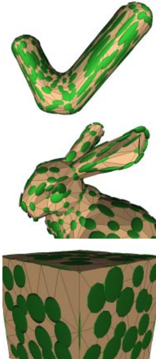
Figure 4.1: Quadric error isosurfaces on three simplified models: blobby “V”, bunny, and the corner of a cube. Note how the ellipsoids follow the local shape of each surface.
