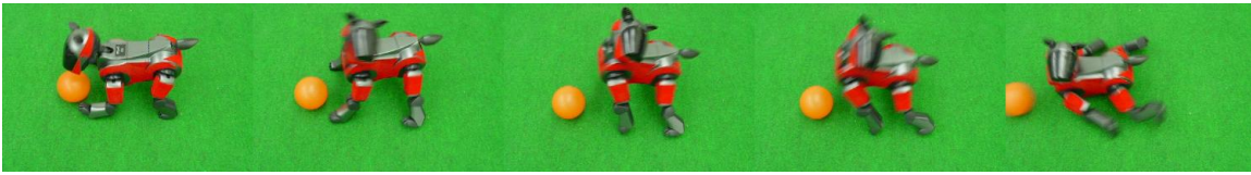
Figure 2.1: The dive kick. By falling onto the ball with its chest, the robot uses the weight of its body to propel the ball forward.
