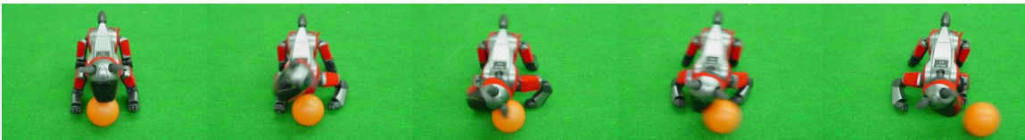
Figure 2.3: Normal head kick. The robot uses the side of its head to kick the ball to either the left or right side, nearly perpendicular to the robot.
