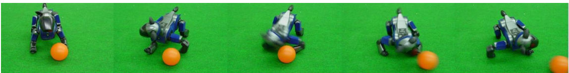
Figure 2.4: Hard head kick. Similar to the normal head kick, this motion also kicks the ball to the side. By swinging the entire body in addition to the head, the robot achieves greater force for a stronger kick.
