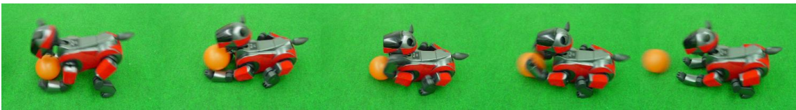
Figure 2.2: The forward arm kick. The robot uses its arms to grab the ball and position it in the middle of its chest. The mouth is opened to keep the ball from settling too close to the chest. The arms are then used to drive the ball forward.
