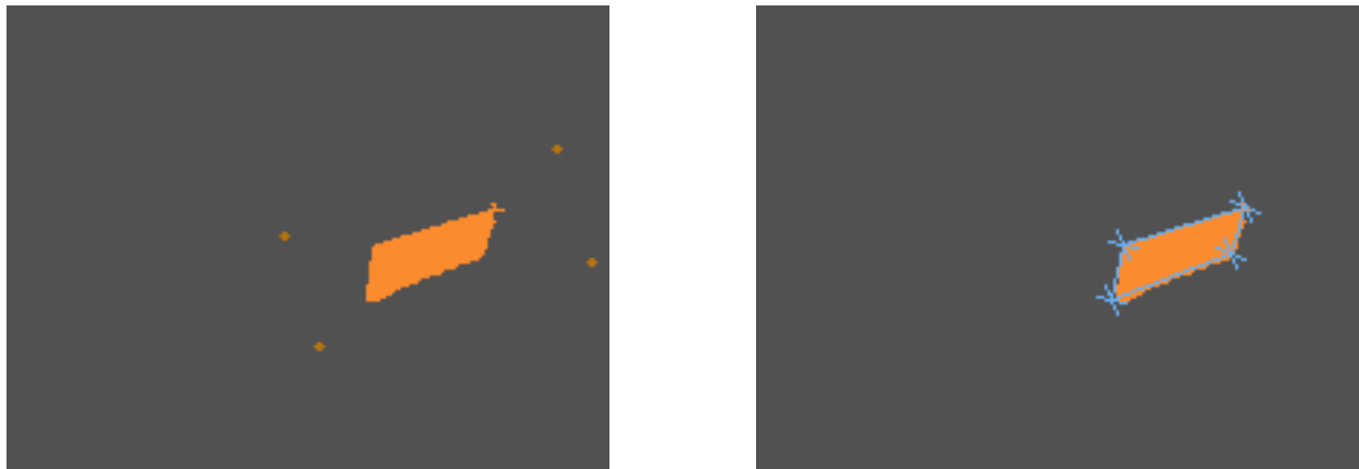
Figure 3: a) Candidate points found for a quadrilateral around this face; b) The converged quadrilateral.
