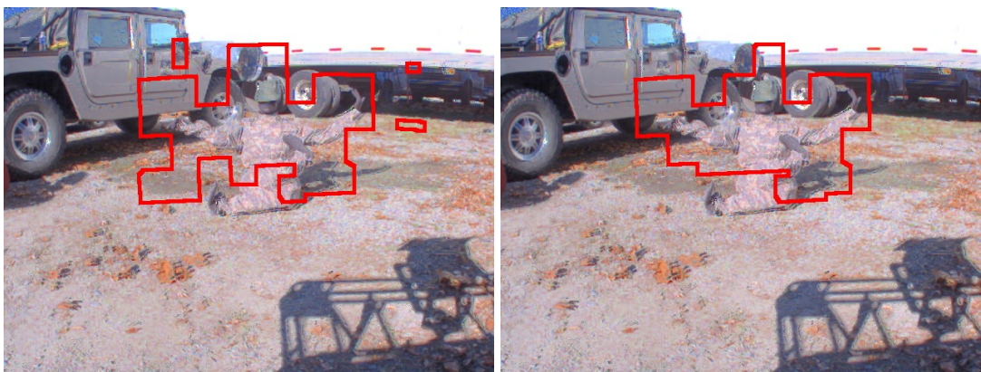
Figure 13: A visualization of change detection without segmentation (left) and with segmentation (right). The red outline is the outline of the changed voxels. The result with segmentation has notably fewer false positives
