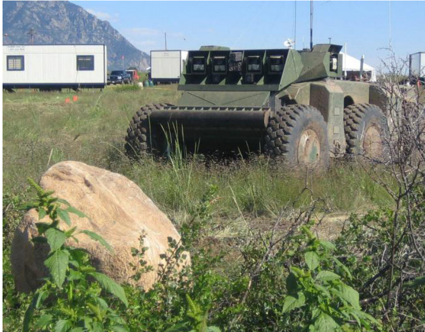
Figure 6: The Crusher vehicle of the UPI program. A majority of the core autonomy system for our platform is derived from that of the Crusher autonomy system.
