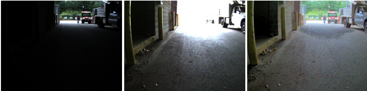
Figure 4: Example output from HDR camera system. An image of low exposure (left) is combined with an image of high exposure (center) to create a single image that is well-exposed for the entire scene (right).
