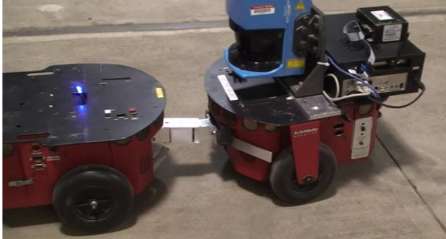
Figure 7 - Prototype recharging hardware. Note the recharging robot on the left and the worker robot on the right.
