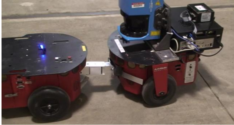
Figure 3 - Pioneer with recharging arm docked with another Pioneer
