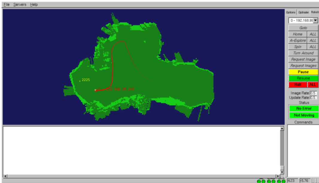
Figure 4 - Graphical user interface showing a robot's location, path, and a map of the known environment. The interface allows for direct control of the robots.
