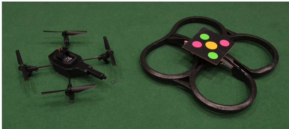
Fig. 1. The quadrotor we used to demonstrate our visualization, alongside its protective hull, which is used for safety when flying indoors. The colored pattern on top is not normally part of the hull; we used it for tracking (see Section 5 ).
