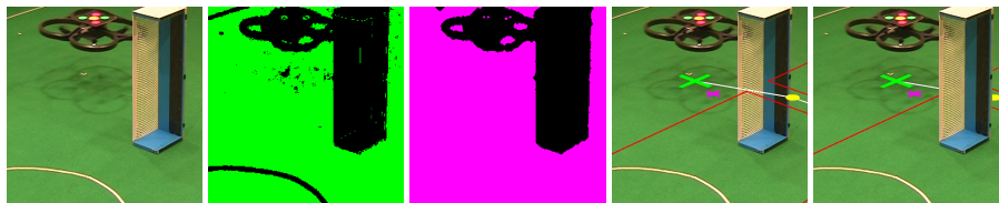
Fig. 4. The stages in processing each frame of a video to overlay the virtual drawings. From left to right: (1) the original frame, (2) the raw green mask, (3) the mask, after morphological operations, (4) the result of drawing without taking the mask into account, and (5) the drawing, masked appropriately.
