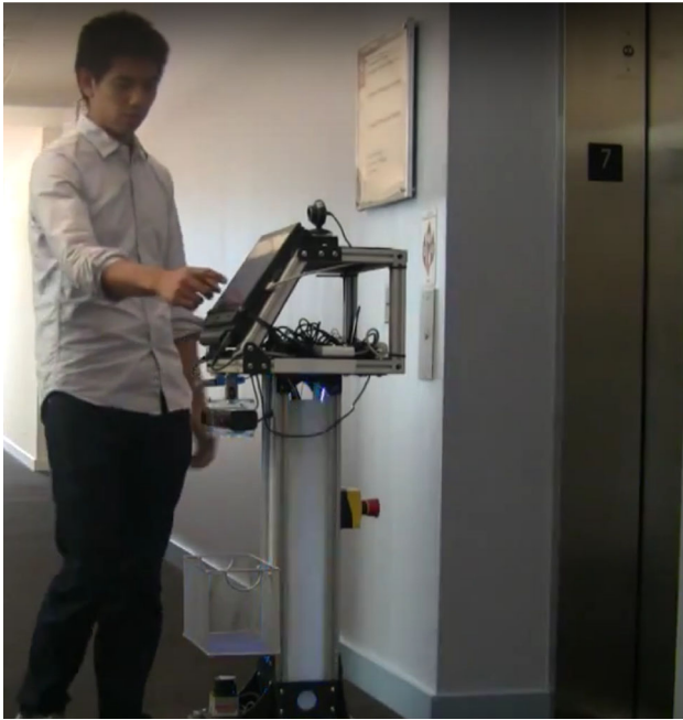
Fig. 3 An example of symbiotic autonomy: CoBot getting help from a human at an elevator
