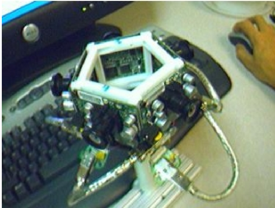
Figure 3: The FDM mount for the five firewire cameras.
