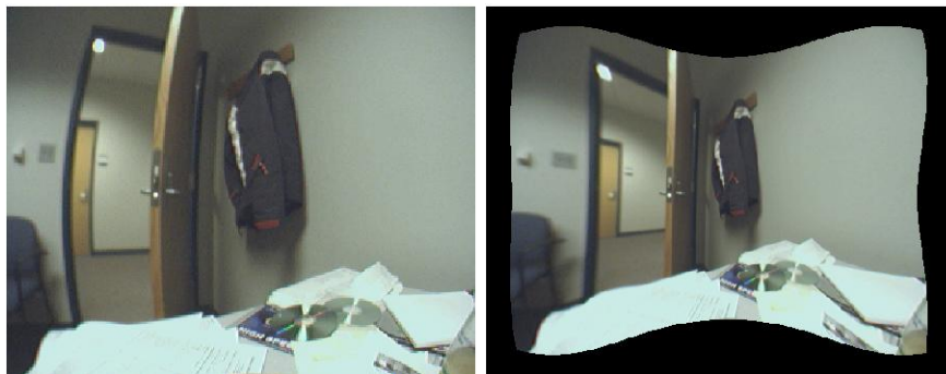
Figure 4: a) Original image b) Corrected image. Straight lines in the world are mapped to straight lines in the image.
