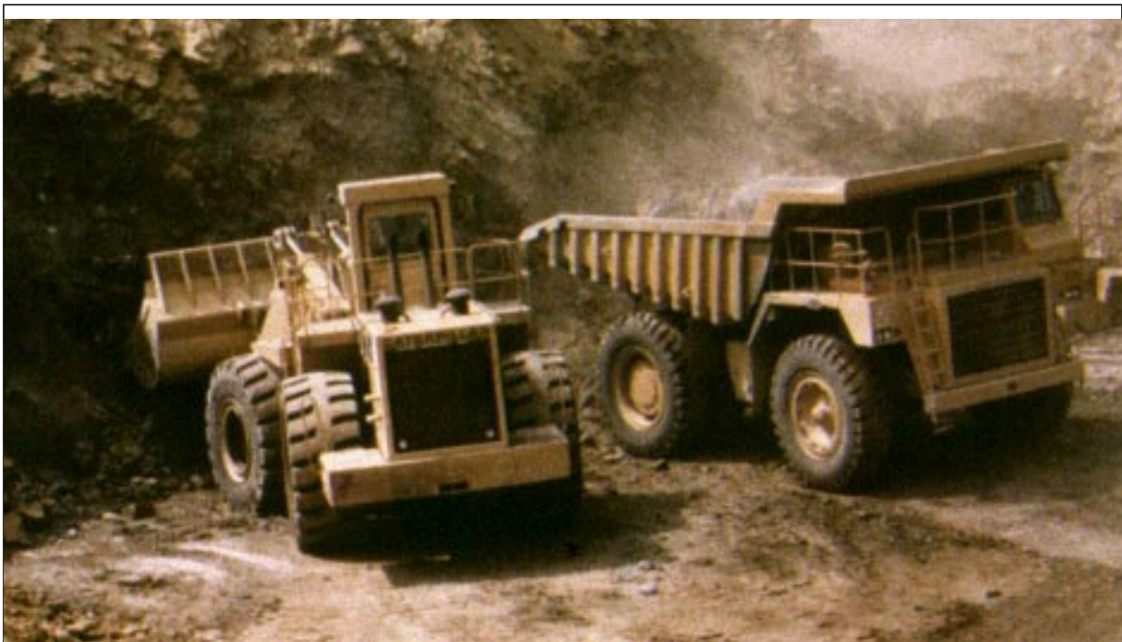
Figure 12: A wheel loader digging next to a truck. The operator is incapable of seeing the material in the bucket during the digging process.
