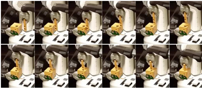
Fig. 12: Snapshots of a robot experiment for a 2D peg-in-hole task.
