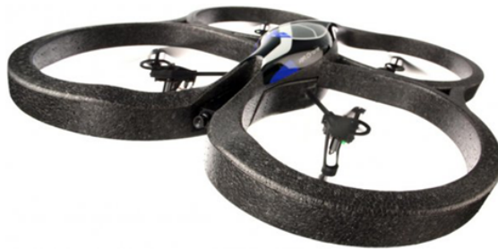
Figure 5.6: The Parrot ARDrone, a cheap commercial quadrotor.
