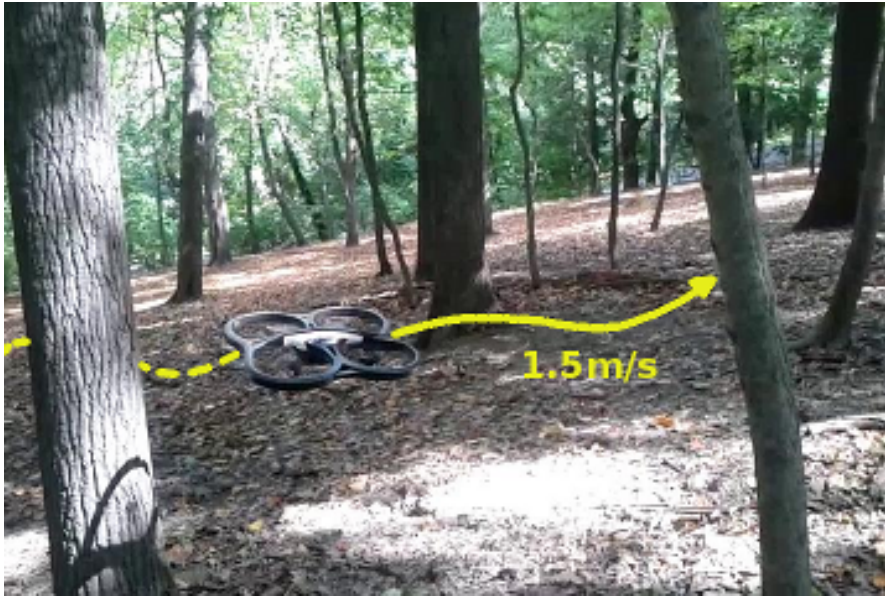
Figure 5.5: Application of DAGGER for autonomous MAV flight through dense forest areas. The system uses purely visual input from a single camera and imitates human reactive control.
