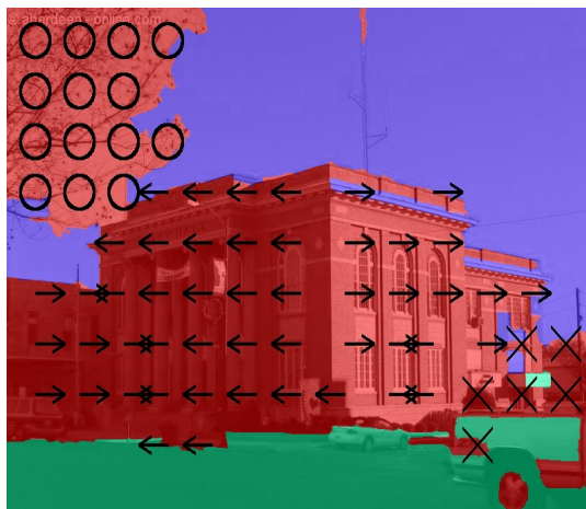
Figure 6.13: 3D Geometry estimation application. Each superpixel is assigned to one of 7 classes: sky, ground, left-perspective, right-perspective, center-perspective, solid or porous.
