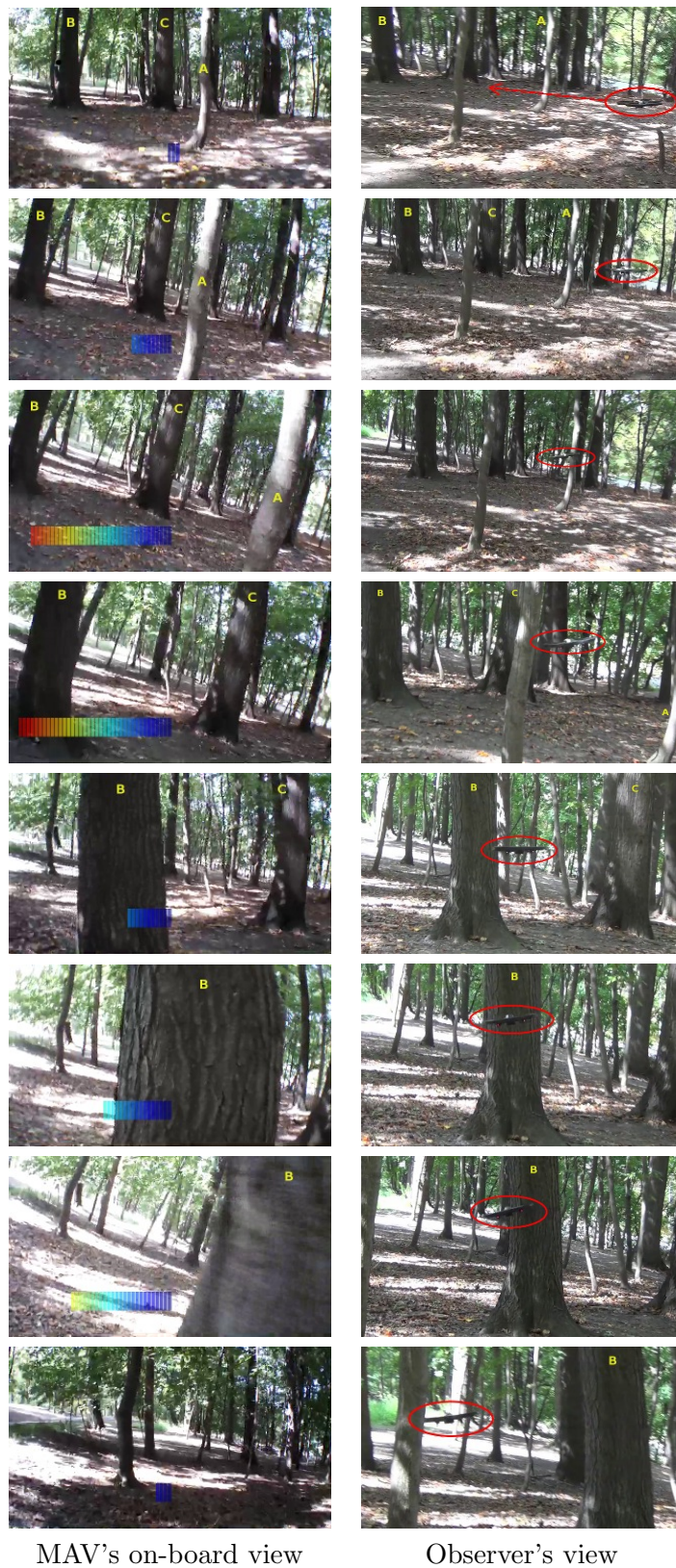
Figure 5.13: Example flight in dense forest. Images ordered from top ( t = 0s ) to bottom ( t = 6.6s ); with color-coded commands issued by DAGGER (in MAV's view). After avoiding tree A (frame 3), drone still rolls strongly to the left (frame 4), in part due to latency. Then tree B is avoided on the left (frame 5-7), rather than on the more intuitive right. Drone prefers this due to the drift feature, as inertia is already pushing it further to the left.
