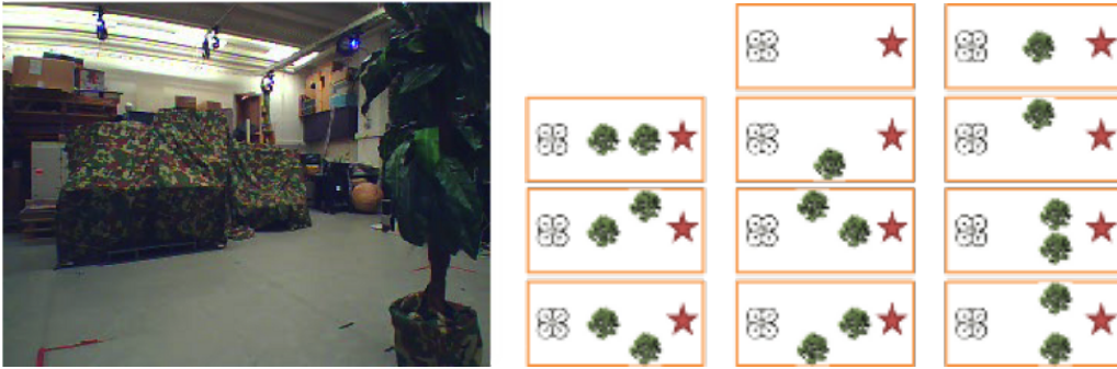
Figure 5.8: Left: Indoor setup in motion capture arena with fake plastic trees and camouflage in background. Right: The 11 obstacle arrangements used to train DAGGER for every iteration in the motion capture arena. The star indicates the goal location.
