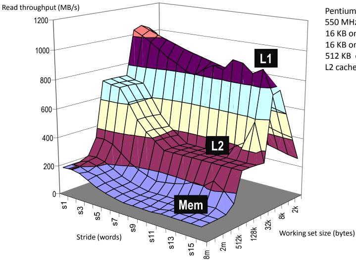
Pentium III Xeon 550 MHz 16 KB on-chip L1 d-cache 16 KB on-chip L1 i-cache 512 KB off-chip unified L2 cache
