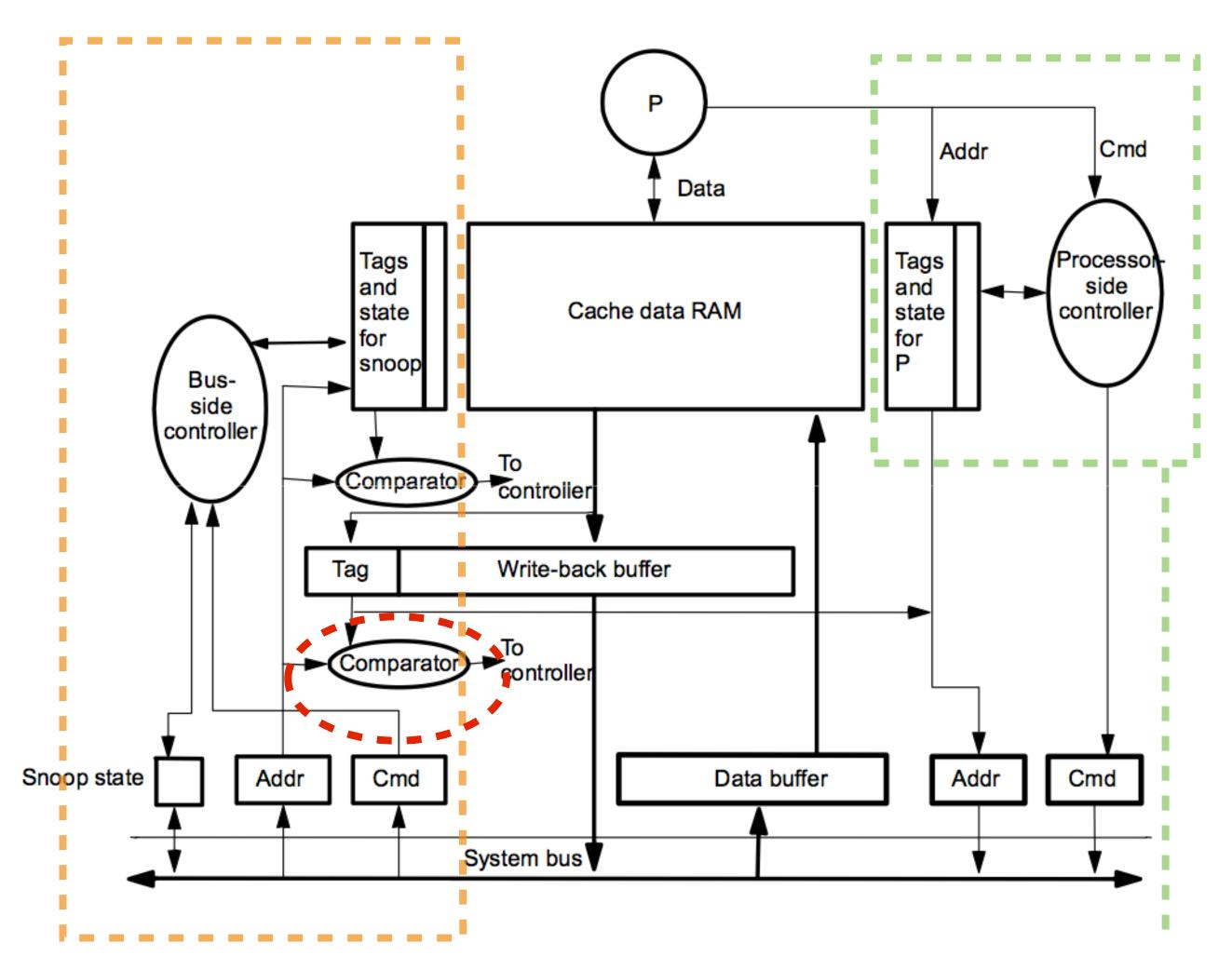
What if a request for the address of the data in the write-back buffer appears on the bus?
