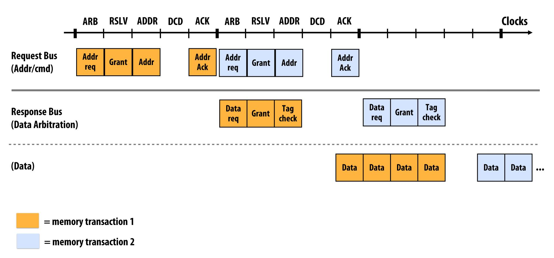
Note: write backs and BusUpg transactions do not have a response component (write backs acquire access to both request address bus and data bus as part of "request" phase)
