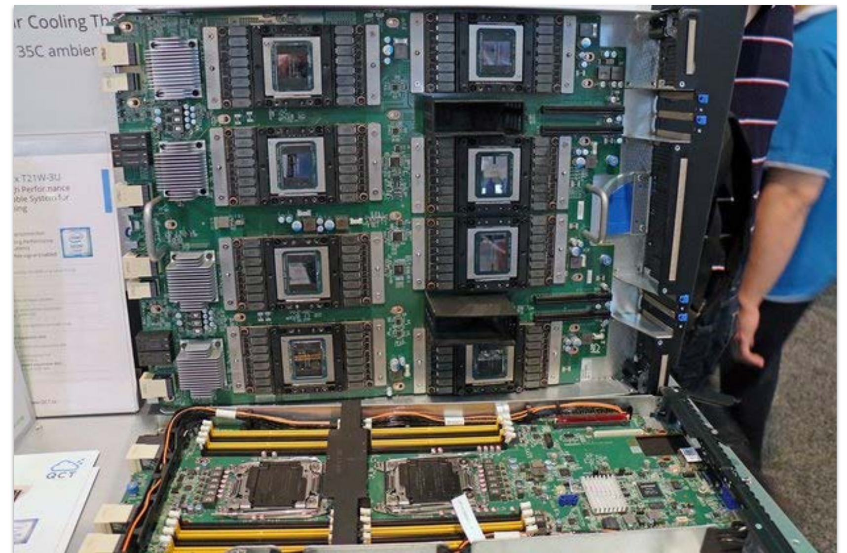
NVIDIA DGX-1: 8 Pascal GPUs connected via high speed NV-Link interconnect
