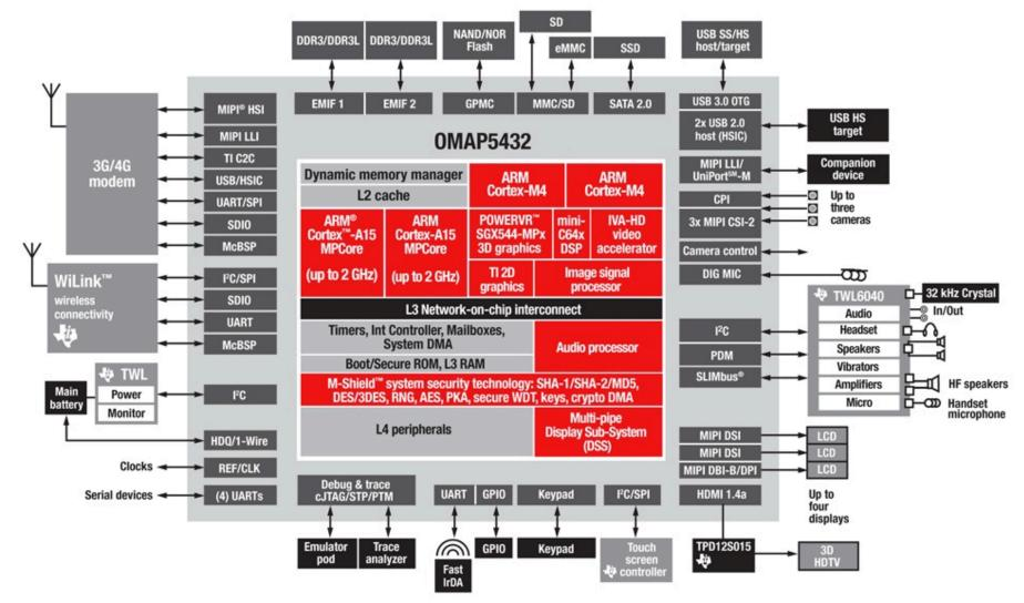
Mobile system-on-a-chip: CPU+GPU+media processing
