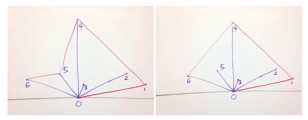
After all the points are processed in this way, we can just add the last segment from  $P_{n-1}$  to  $P_0$ , to close the polygon, which will be the convex hull.
