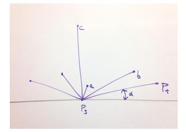
All the other points must be to the left of segment  $(P_s, P_t)$ . We can continue this process to find the point  $P_u$  which is the one with the smallest angle with respect to  $(P_s, P_t)$ . This process is continued until all the points are exhausted. The running time is O(n) to find each segment. There are O(n) segments, so the algorithm is  $O(n^2)$ .
