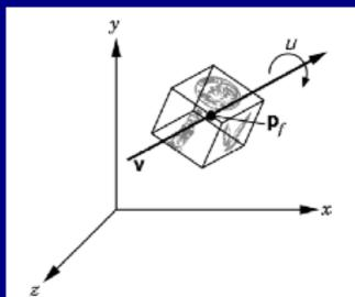
Rotation angle and line about which to rotate
