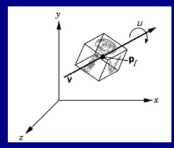
Rotation angle and line about which to rotate
