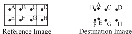
Figure 10: A fold-over configuration. Samples A and E are on the “wrong” side of samples B and F .
