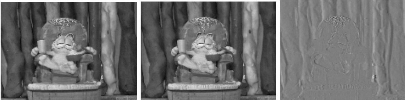
Figure 1: Representative images from the "Garfield" image data set, reduced from color to monochrome only for illustration. (Above) The left image is a left eye view, the center image is a right eye view, and the right image the difference between them. Interocular separation is 40 mm; center-of-image compensation results in on-screen disparities that are nevertheless small, as can be seen in the difference image. Readers who can parallel "free view" should easily see the left and center image pair in stereo. (Below) Pictures of the "Garfield" scene with telephoto (left), normal (middle), and wide-angle (right) lenses at corresponding long, intermediate, and short distances from camera to scene. Distance and focal length are adjusted so that the each image is about the same angular size on viewing. But notice the relative "flatness" at the left, the relative "depth" at the right.
