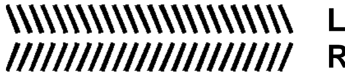
Figure 4: Two states (R, L) of louver filter. Looking up from this caption toward the filter, in the R state the bias favors the right eye, in the L state it favors the left eye.
