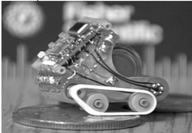
Figure 4: Sandia's toy-balloon treaded Microrobot. The out-of-focus scale in the background is in units of 1/16 inch, equal to 1.5875 mm. [18]
