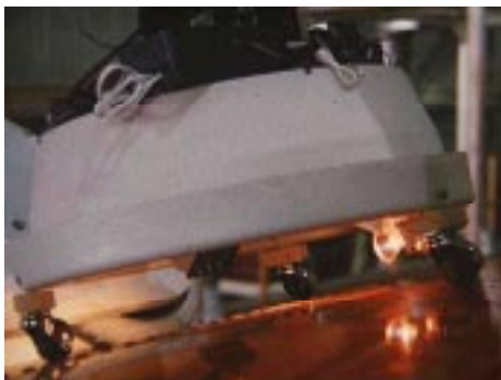
Figure 3: Close-up of CIMP’s sensor pod. Stereoscopic macro camera looks at the surface at a 45 degree angle. Flood and grazing angle spot lighting are remotely controlled. Grazing angle illuminator rotates +/- 150 degrees around the camera pointing direction.
