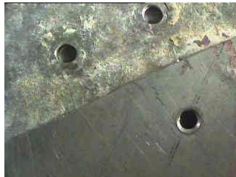
Figure 5: Typical corroded region on aircraft skin material. Corrosion appears above the diagonal. Potentially confounding features such as dirt and paint splashes appear below the diagonal.
