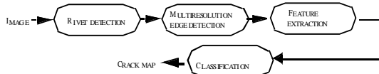
Figure 1: Image processing pipeline for crack detection. Pipeline for surface corrosion detection is similar. Main difference is in the classification step: fuzzy logic is used for cracks, neural net for corrosion.
