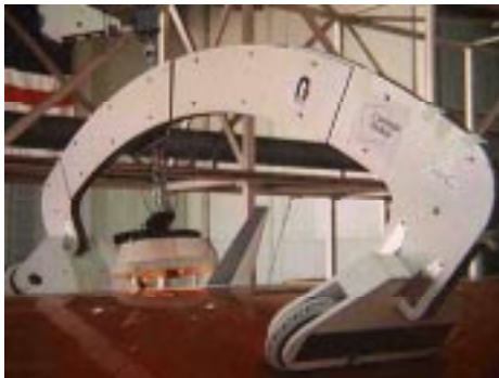
Figure 2: CIMP, the Crown Inspection Mobile Platform. It is battery operated, wirelessly controlled, and has two video download channels.
