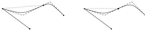
Figure 14: Secant length (dotted line) near small angles can be adjusted using the knot sequence of boundary B-splines (deBoor controls shown dashed).
