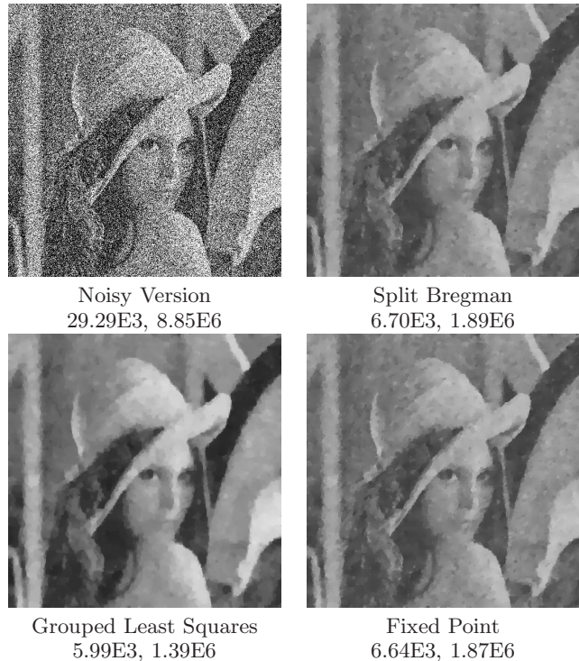
Figure 1: Outputs of various denoising algorithms on image with AWGN noise. Starting from top left in clock-wise order: noisy version, Split Bregman [18], Fixed Point [30], and Grouped Least Squares. Errors listed below each figure from left to right are L_2 and L_1 norms of differences with the original.
