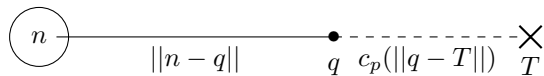
Figure 2. Given a robot at position n and a perception target T in a scenario without obstacles, the optimal sensing goal position lies in the straight line connecting those two points.
