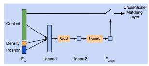
Figure 2: The gating network architecture.
