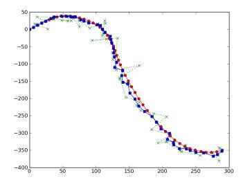
Figure 1: The blue line is the expected path, the green paths are the observed path from the two towers given in the files, and the red path is the true trajectory of the UAV. You are not given the data for the red path.
