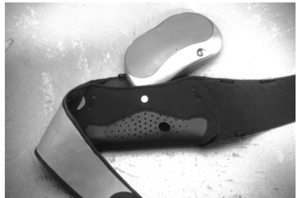
Figure 7. Navigator 2 wearable computer for aircraft maintenance engineers integrates a humanistic form language with attachment guidelines, placement guidelines (small off the back) and aesthetic, perceptual, and sensory informed use of materials.
