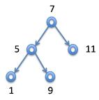
Even though, locally, the key of the left node is always smaller and on the right is always bigger, the node with key 9 is in the wrong place and we would not find it with our search algorithm since we would look in the right subtree of the root.
