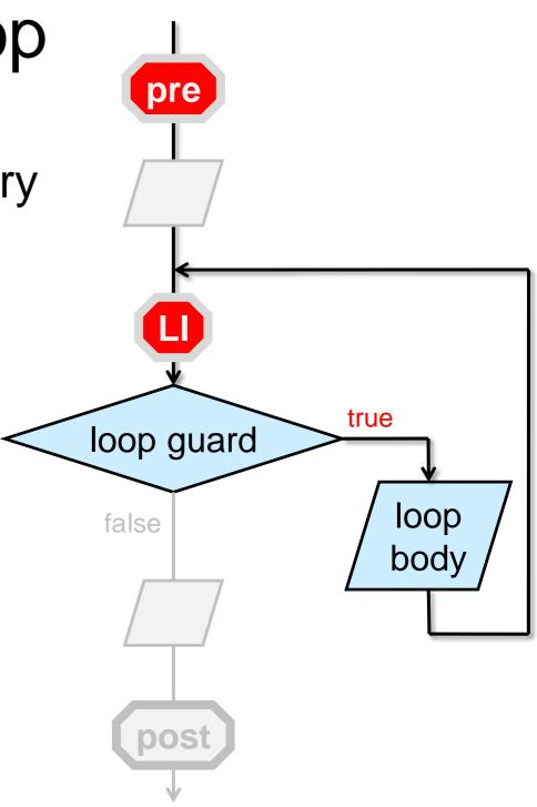
**EXIT:** the loop invariants and the negation of the loop guard imply the postcondition
